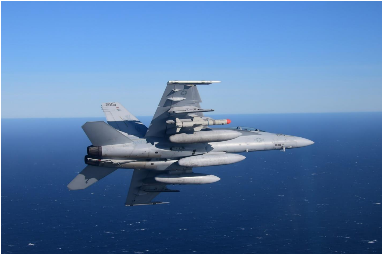
November 2015 – An F/A-18 armed with a Harpoon Block II+ missile during a free flight test at Point Mugu's Sea Range in California. (U.S. Navy photo)[/caption]
