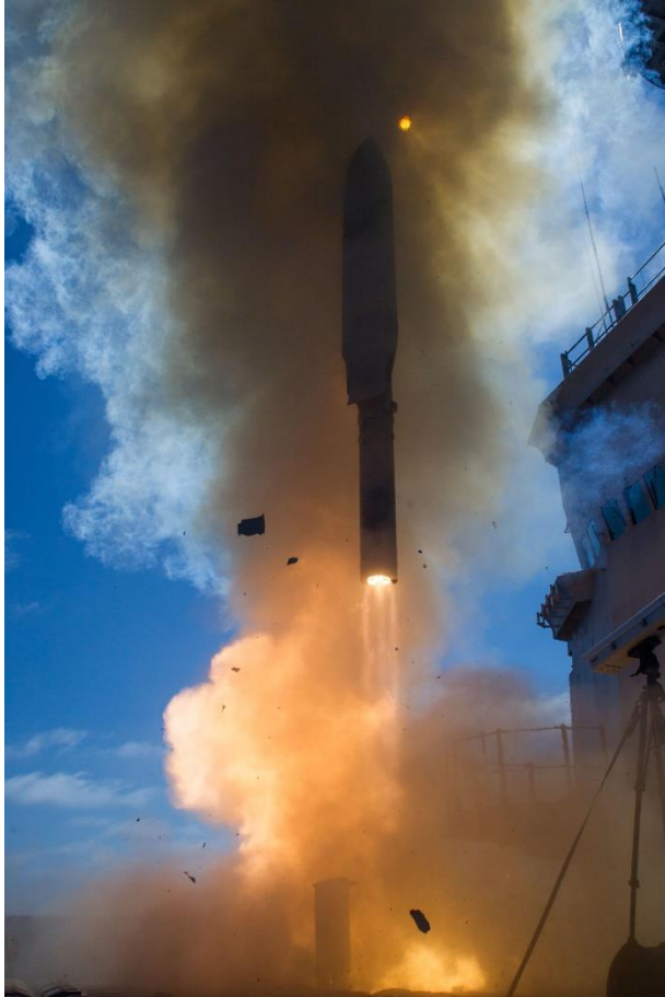
A July 2016 test of the LRASM from a MK-41 launcher on the Navy's Self Defense Test Ship. (Lockheed Martin photo)[/caption] (Change photo)
