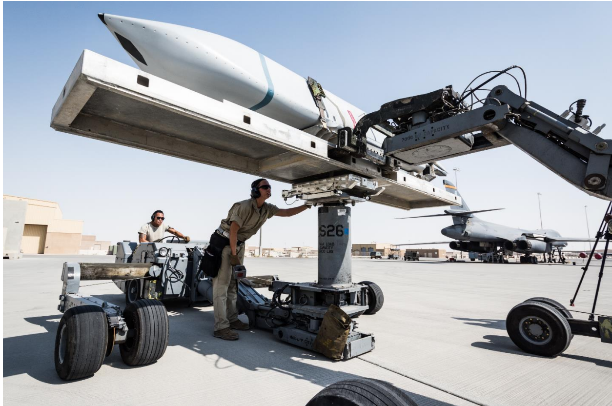
Sept. 13, 2018 – An inert AGM-158A Joint Air-to-Surface Standoff Munition (JASSM) being used in a training exercise on a B-1B Lancer at Al Udeid Air Base, Qatar. (U.S. Air Force photo by Tech. Sgt. Ted Nichols/Released)[/caption]
