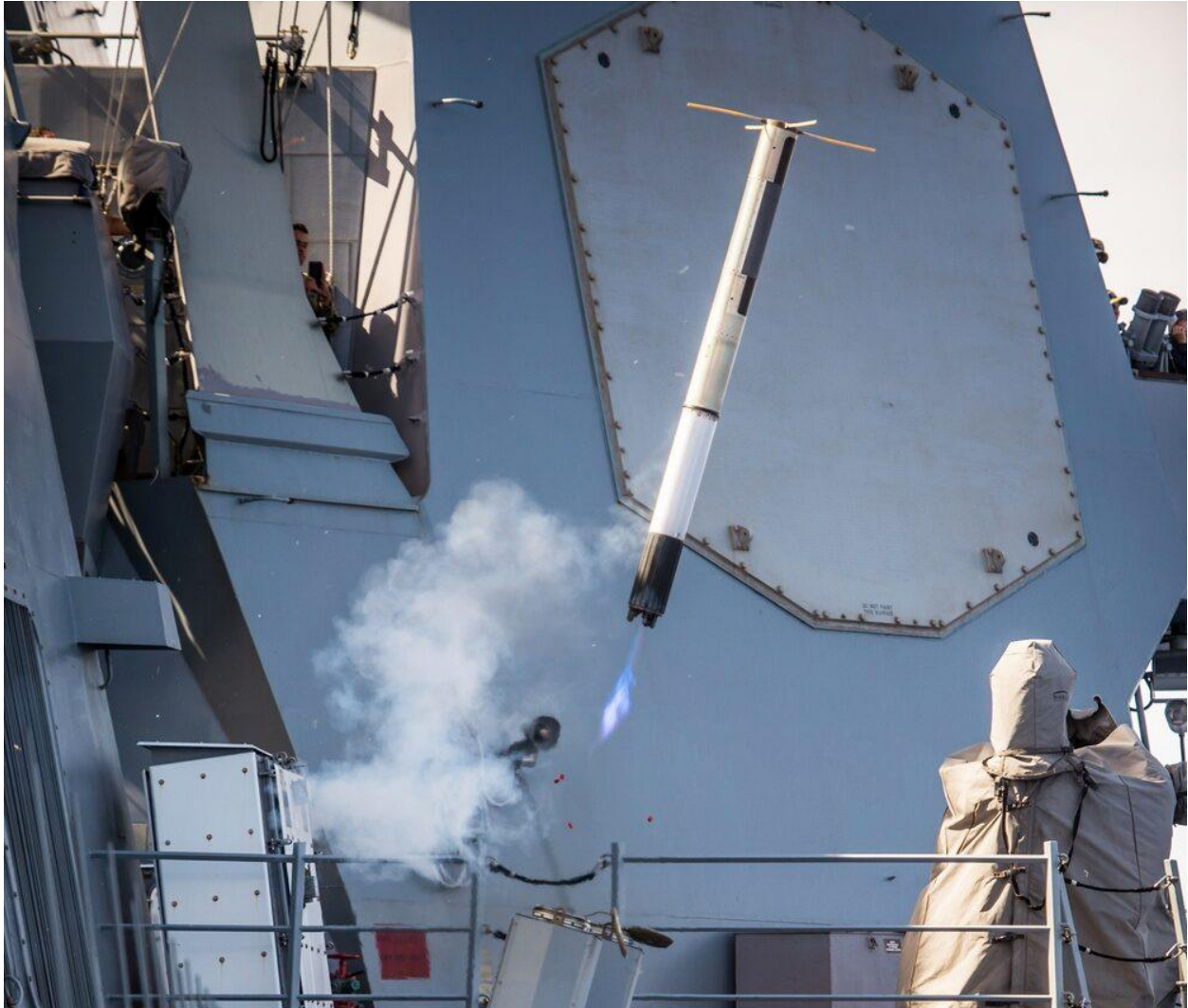
PACIFIC OCEAN (July 11, 2018) – The guided-missile destroyer USS Dewey (DDG 105) launches an electronic decoy cartridge from an MK-234 Nulka Decoy Launching System while underway. (U.S. Navy photo by Mass Communication Specialist 2nd Class Devin M. Langer/Released)[/caption]
