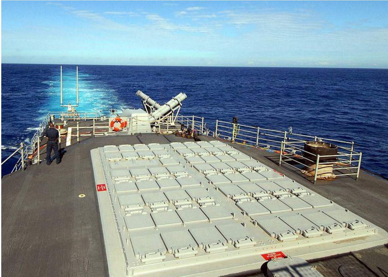
PACIFIC OCEAN (Feb. 18, 2008) Note the four Harpoon missile launchers in the background and the 64 vertical launch cells in the foreground. Original caption: Seaman Robert Paterson, of Norgo, Cal., stands watch next to the aft vertical launch missile platform on the fantail while underway on the guided-missile cruiser USS Lake Erie (CG 70). (U.S. Navy photo by Mass Communication Specialist 2nd Class Michael Hight)[/caption]
