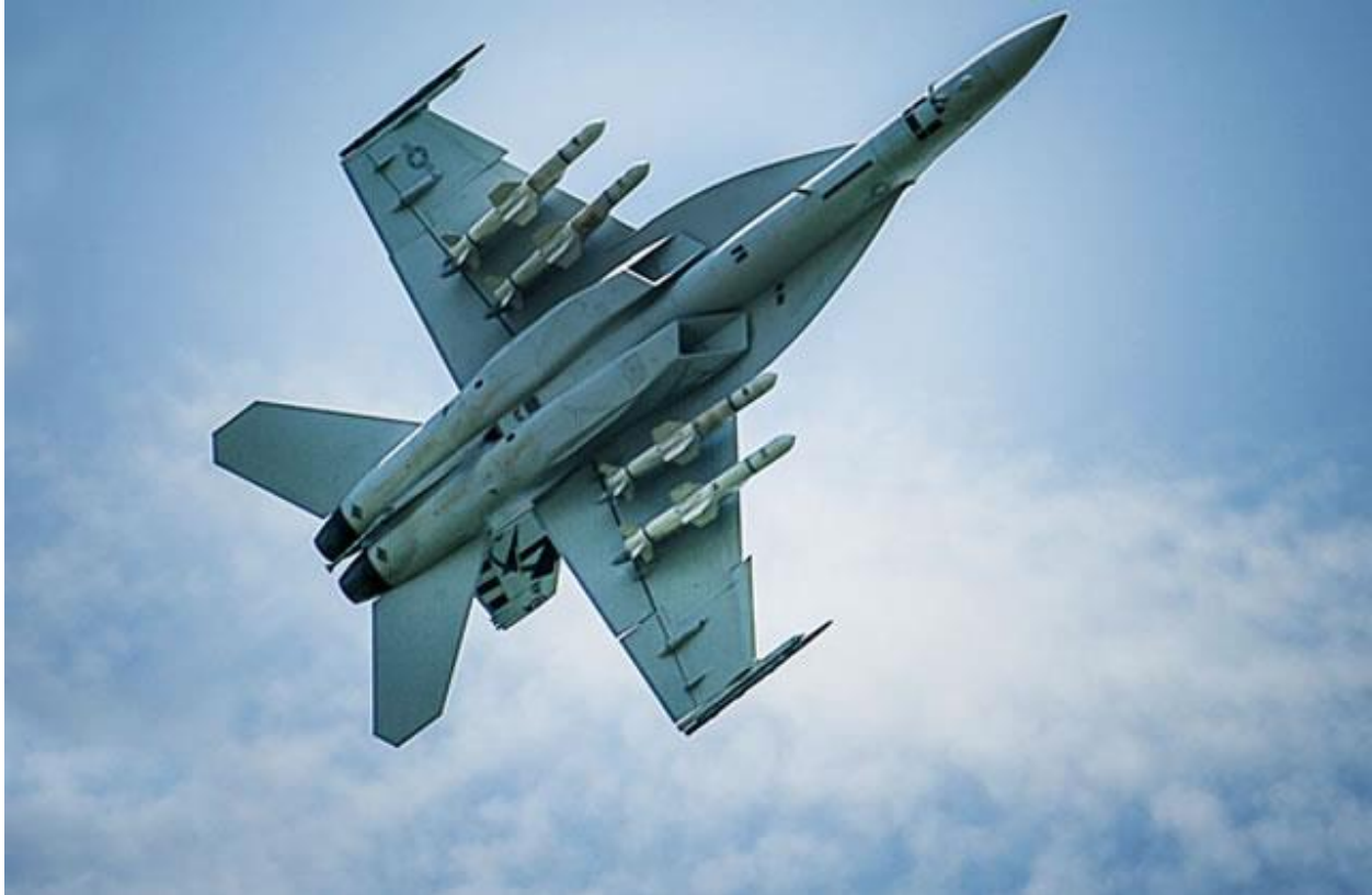
An F/A-18F Super Hornet from U.S. Navy Strike Test VX-23 in flight with four Harpoon anti-ship missiles. (Boeing photo)[/caption]
