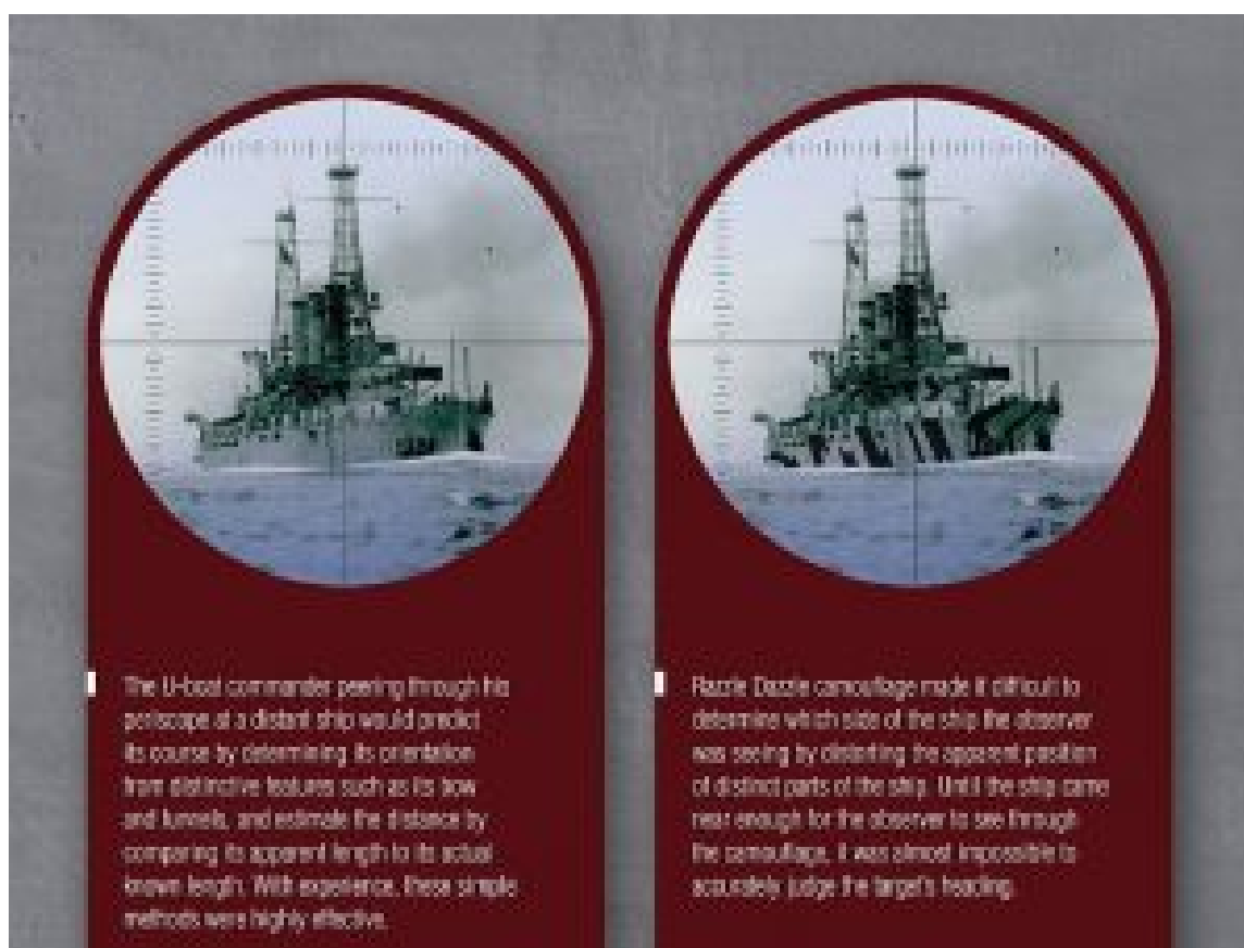
Dazzle was intended to deceive U-boats about the ship's speed and course/U.S. Navy File Image
